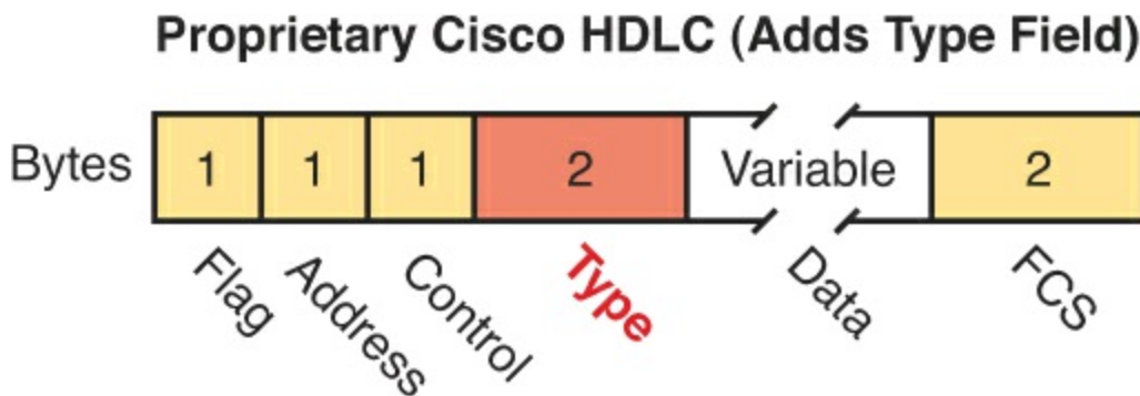
Figure 12-9. Cisco HDLC Framing
