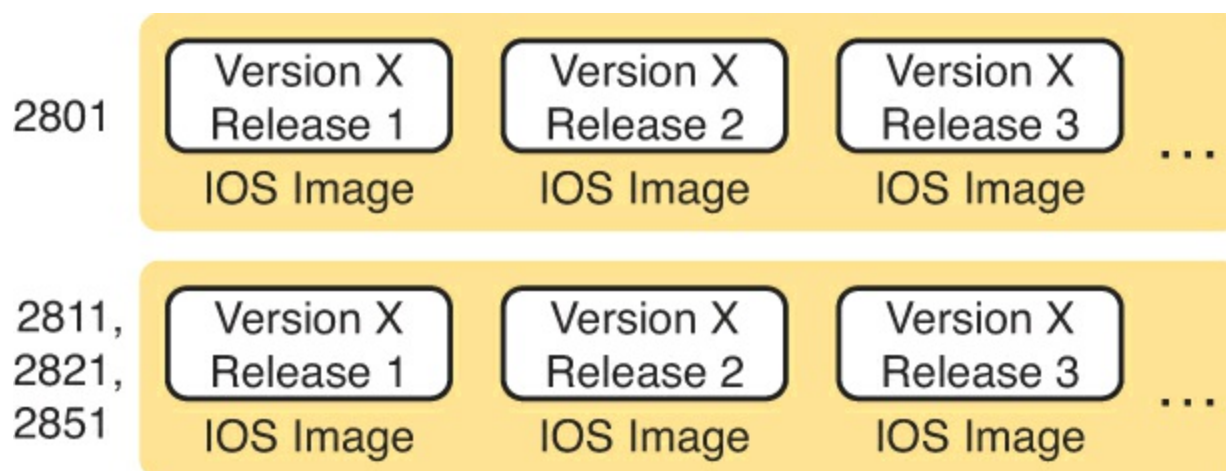
Figure 21-1. IOS Images per Model or Model Series, per Version/Release
