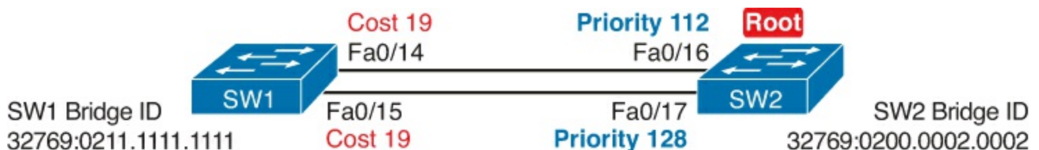
Figure 2-9. Topology Required for the Last Two Tiebreakers for Root Port
